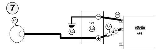
Basic 12VDC Vehicular Battery Connection. See Pg.8.
